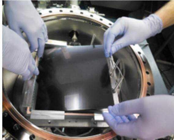
**Step 3:** Position Sb coated window for sealing
