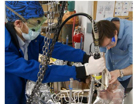
**Step 6:** Pinch seal copper tube
