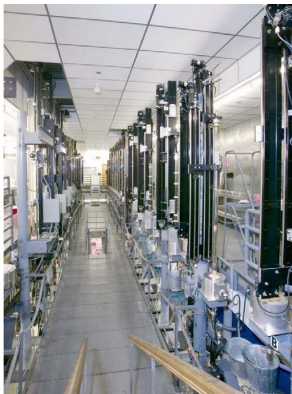
Figure 23. The capillary drawing facilities at Incom. The capillaries are cut, stacked and fused into a solid block, which is then sliced into wafers that are ground, polished, and trimmed to become the MCP substrates.
