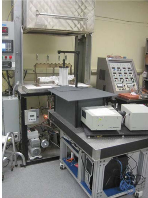
Figure 28. The commercial Photocathode Deposition facility, purchased from Burle/Photonis, installed in the High Energy Physics Division at ANL. The instrumentation used for measuring film thickness and quantum efficiency is in the foreground.
