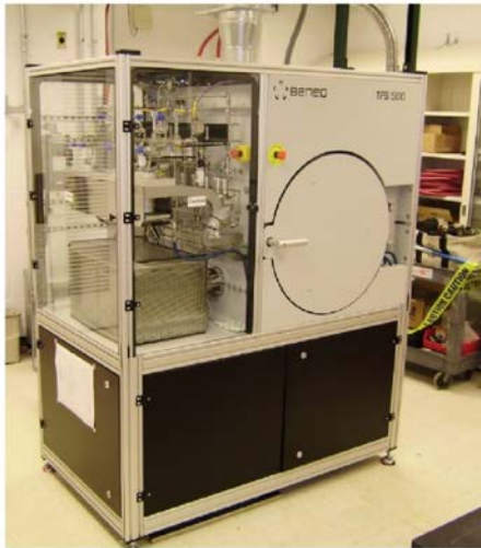
Figure 25. The Beneq Atomic Layer Deposition facility installed in the Energy Systems Division at ANL, used to functionalize the Incom capillary plates with resistive and secondary-emitting layers. The precursor flow path required extensive modification in order to establish uniformity over the 6.5 m 2 surface area of each capillary plate.
