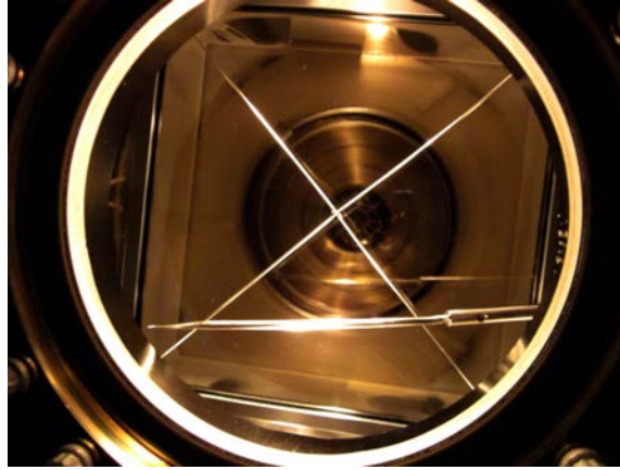
Figure 13. A K_2NaSb photocathode synthesized on a stand-alone LAPPD window in the large fabrication tank at the Space Sciences Laboratory [36, 18].
