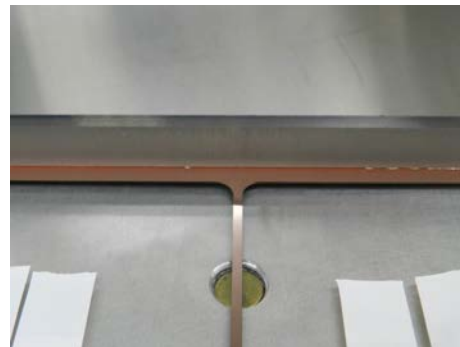
Figure 12. A glass LAPPD™ package with a hermetic indium 'flat' seal between the glass sidewall and the glass top window under test. Right: A close-up of the indium flat seal, taken through a top window with no photocathode. The photo shows the NiCr metalization on the top surface of the sidewall; a Cu layer is visible where the indium has not taken it into solution. The Cu/NiCr "finger" extending towards the bottom of the frame is for distribution of current towards the center of the cathode.
