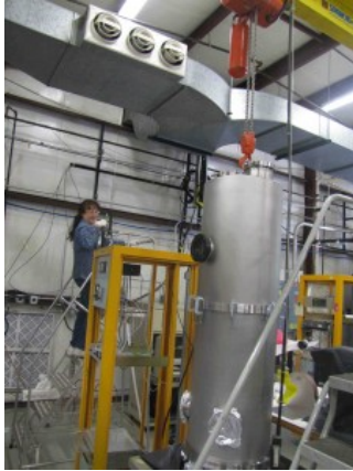
Figure 24. Left: The Fermilab UHV evaporation facility constructed to deposit NiCr electrodes on the top and bottom surfaces of LAPPD™ capillary wafers; Right: A chart of the number of wafers metalized on both sides at the Fermilab evaporation facility versus time.
