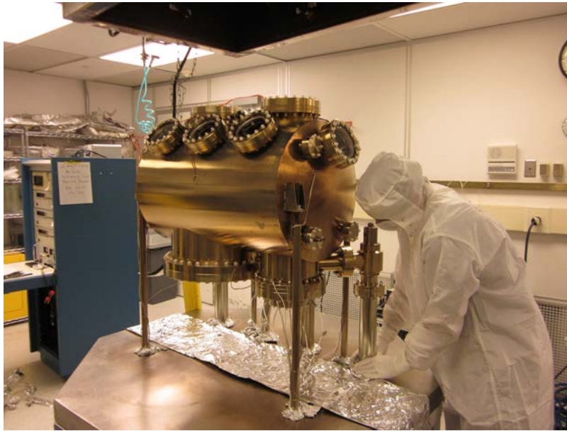
Figure 26. The UHV photocathode and detector assembly facility constructed for LAPPD at the Space Sciences Laboratory, University of California, Berkeley .
