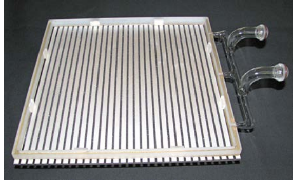
Figure 11. A glass module base assembly showing the microstrip anode [17], and the glass frit joint between the glass sidewall and the anode [35]. The two ports on this assembly are specific to the Demountable test facility at the Argonne Advanced Photon Source, in which the module is sealed with an O-ring and the cathode is a thin aluminum layer [30, 3]. (credit: Joseph Gregar, ANL Glass Shop).
