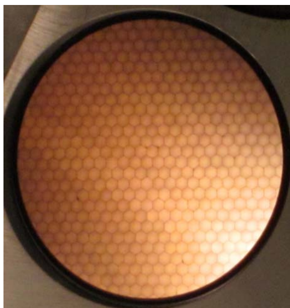
Figure 4. 33 mm borosilicate substrate MCP with ALD and NiCr electrodes, 20 \mu\text{m} pores, 65% open area. Backlit photo.
