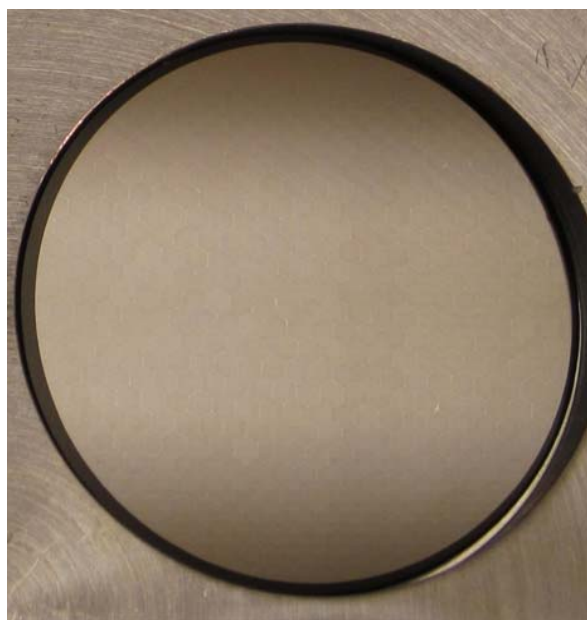
Figure 3. 33 mm diameter, borosilicate substrate MCP with ALD layers and NiCr electrodes, 20 \mu\text{m} pores, 65% open area.
