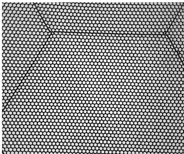
Figure 1. 200 mm square borosilicate micro-capillary substrate, magnified section, 20 \mu\text{m} pores, 65% open area.
