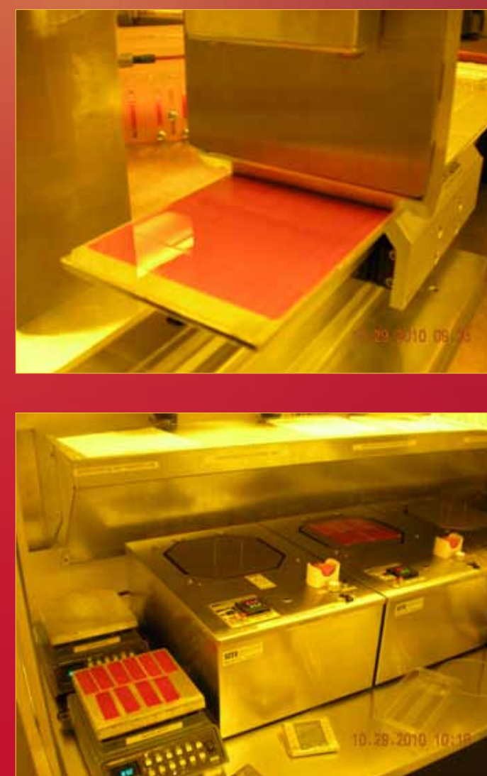
Continuous slot-coating of XP SU-8 Magenta.
