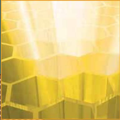
Microcapillary plates are dense arrays of flow-through glass capillaries with large cross-sectional areas and unlimited length to diameter ratio.
