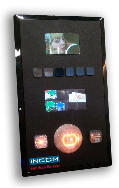
Incom's Fused Fiber Optics Up the Stakes for Gaming Displays: This vertical monitor showcases innovative polymer/fused fiber optic-enabled displays and buttons, each with unique geometric, transmission and image characteristics. <a href="www.incomusa.com">www.incomusa.com</a>
